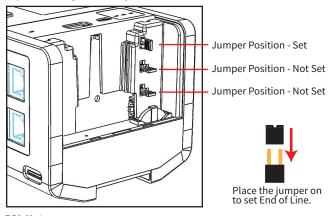
**EOL Note:** In this example, the Omni C20 & Omni C40 and the last REM require EOL jumpers to be set.
